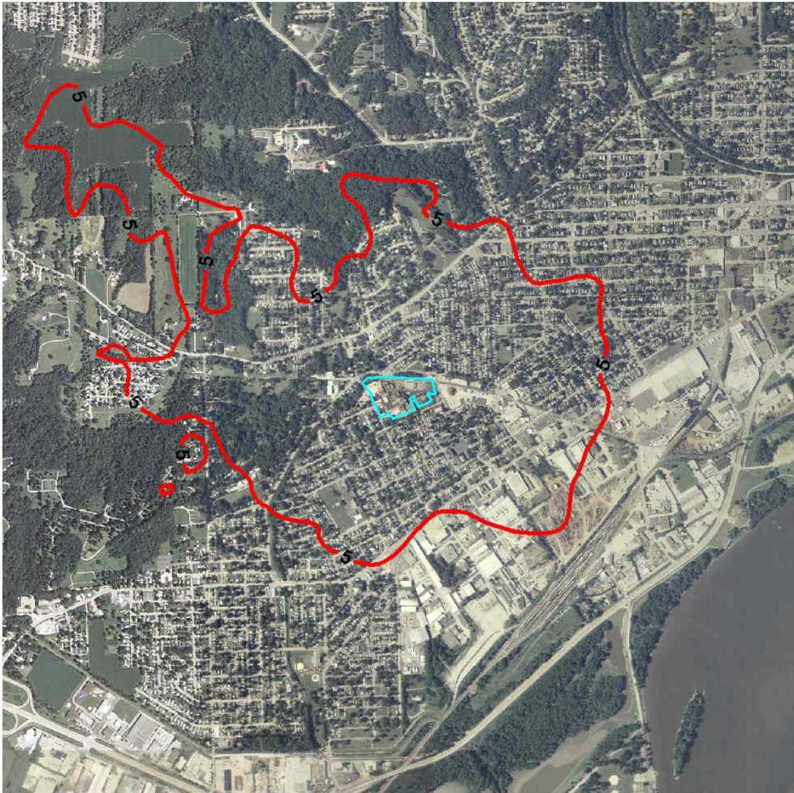
Figure 26. Location of 5 \mu\text{g}/\text{m}^3 Blackhawk Foundry isopleth- base case and completion of Phase 1.
